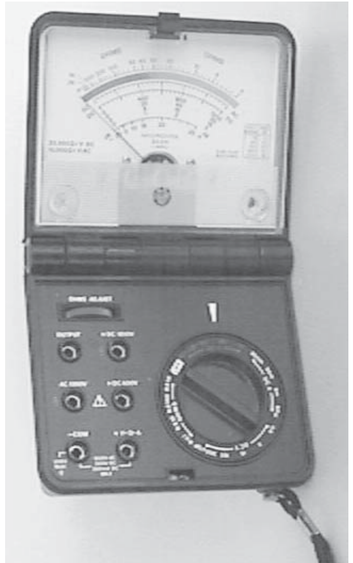
FIGURE 6-5 Volt-ohm milliammeter. (Courtesy of BET Inc.)
